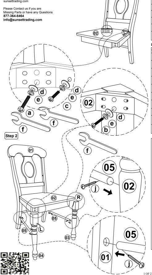
Code Figure Part Qty. Back Frame 1 (01) TR (02) 1 Seat ⋸ 1 (03) Front Leg (R) 1 (04) Front Leg (L) 2 (05) ۵ Side Stretcher (06) Arm (R) 1 100 (07) 1 Arm (L)
